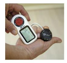
2) Then, put the iBike over the mount and twist it clockwise onto the mount. From the back side it will look like this when properly connected:
